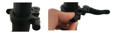
Open the seat post clamp and turn the adjustment knob. Turning left loosens the clamp, turning it clockwise tightens the clamp.
