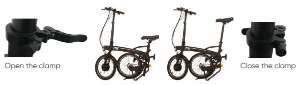
CAUTION! Do not extend the seat post beyond the maximum height indicated on the seat post itself. This marking is located on the front of the seat post, facing the handlebars.
