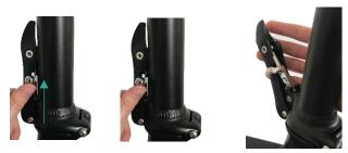
With an open clamp, you can easily fold your handlebars:
